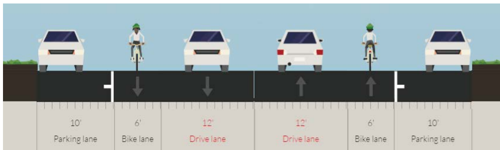
Figure 1 - Existing cross section of Allens Avenue between Indiana Avenue and Ellenfield Street
