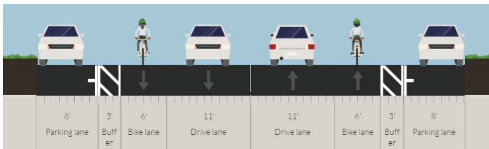
Figure 2 - Recommended cross section of Allens Avenue between Indiana Avenue and Ellenfield Street
