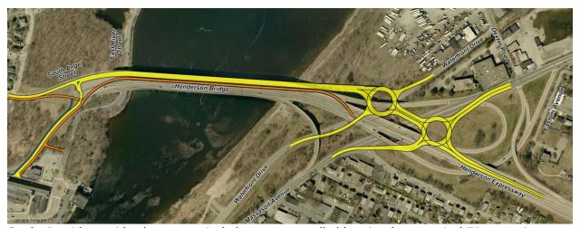
On the Providence side, the concept includes an uncontrolled (no signal or stop sign) T intersection near the foot of the bridge at the intersection of the bridge and South Angell Street. An alternative concept (below) includes a small single-lane roundabout, which could potentially do more to slow down traffic coming off the bridge toward South Angell Street than the uncontrolled T intersection currently proposed.
