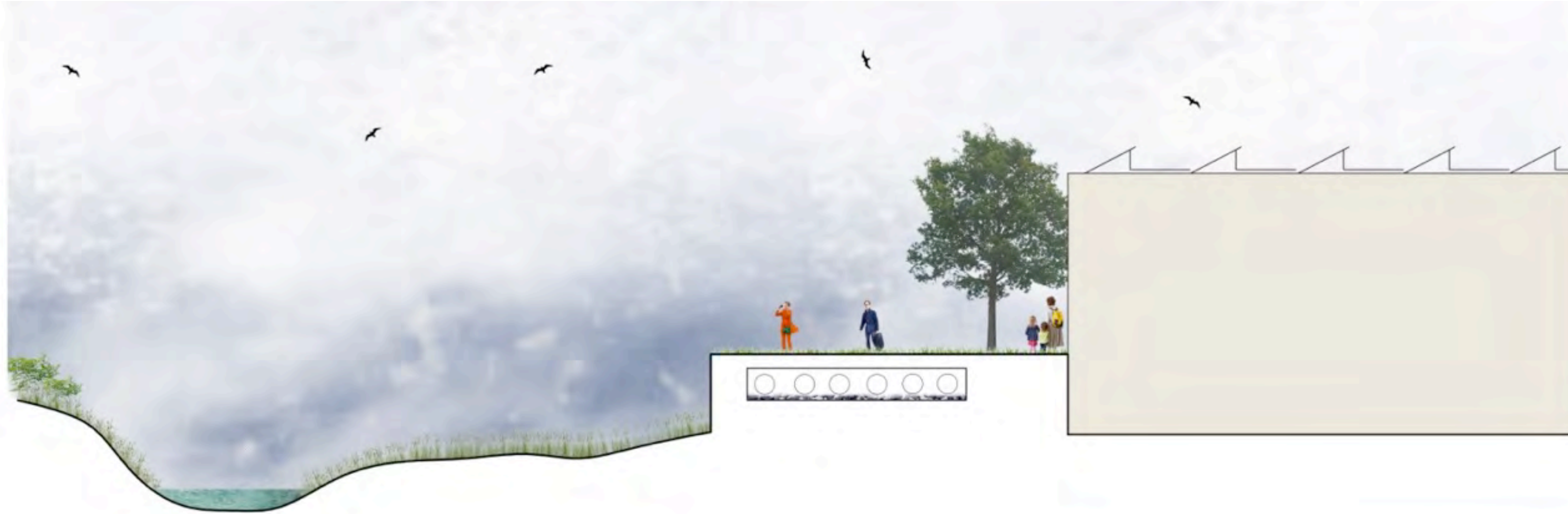
Fill Against Building with Stormwater Management
