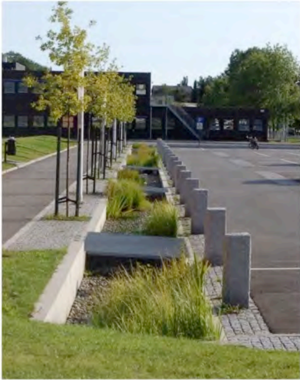
Risenga Idrettspark, Norway - Curbless Parking lot with Bioretention Crossed by Foot Bridges
