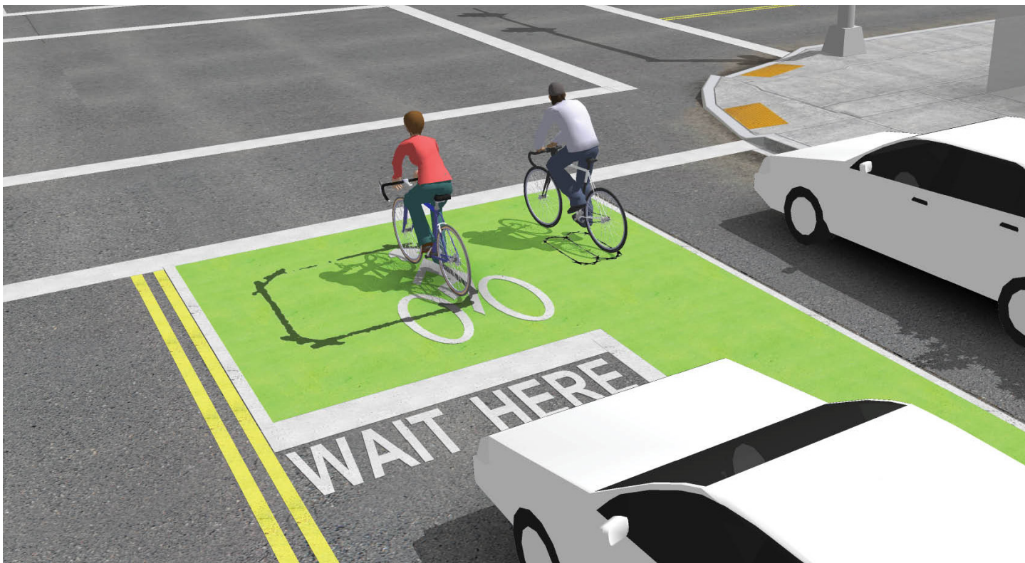
Signal Detection and Actuation - Detection in Bike Lane and Bike Box. Source: NACTO.
