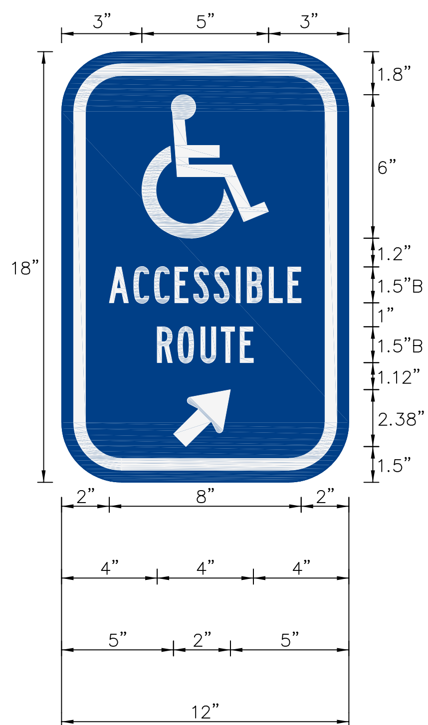
SP-1L/R ACCESSIBLE ROUTE SIGNS (NOT TO SCALE)
