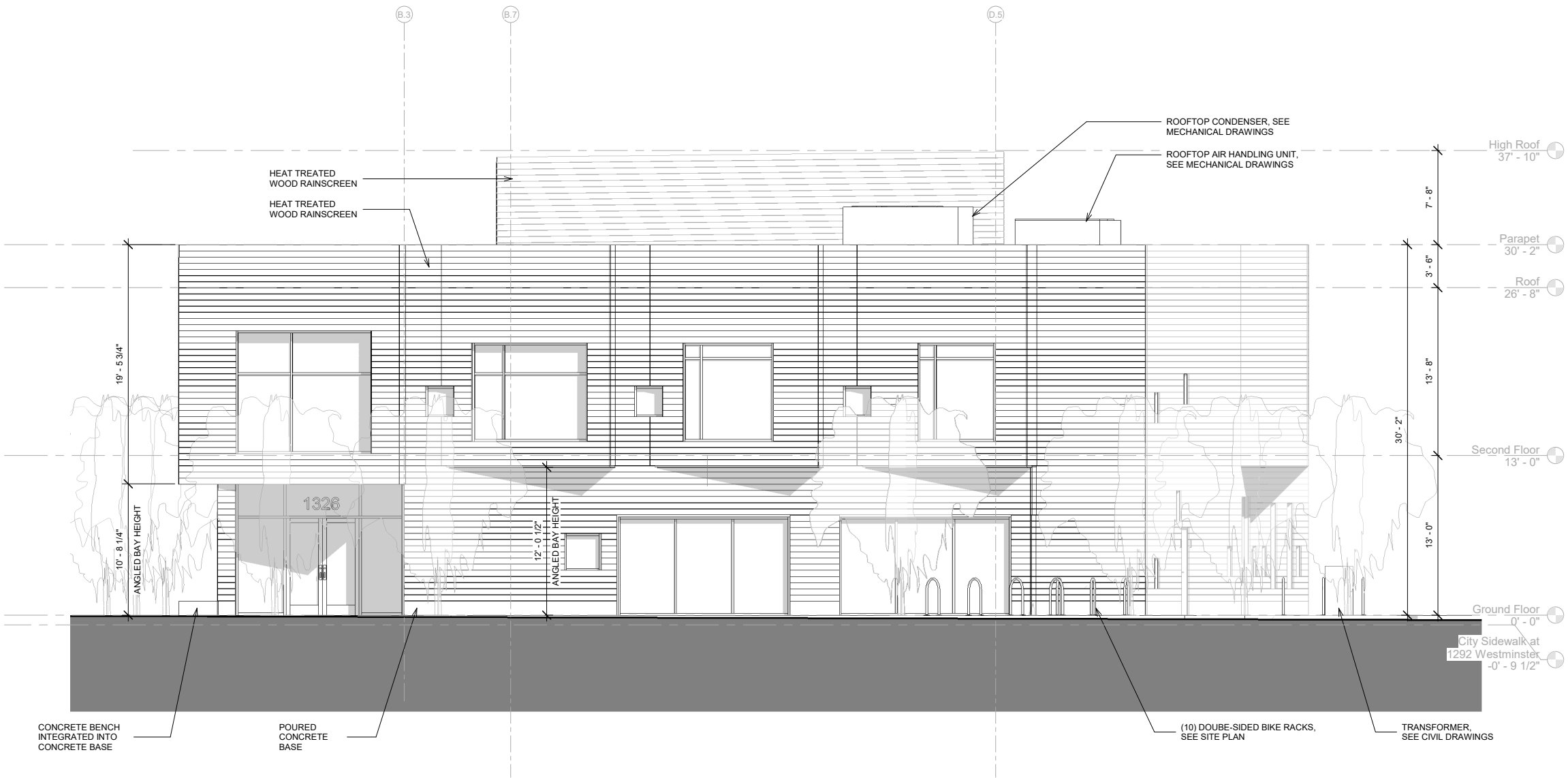
1 EXTERIOR ELEVATION - WEST 3/16" = 1'-0"
