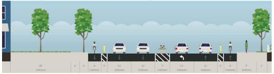
O Charles Street between Orms St and the northern end of 125 Charles St should be restriped to eliminate one vehicular travel lane and install separated bike lanes on each side. In addition, the southbound-to-westbound slip lane should be narrowed, with a separated bike lane on its right-hand side, as pictured below:
