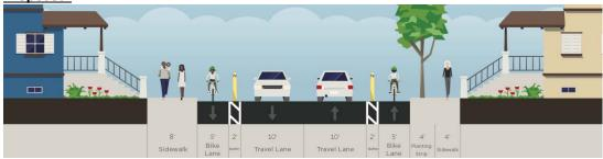
Between Wyndham St and River Ave, a similar configuration should be restriped, but due to the narrower width, the buffers should be omitted (5 ft bike lane, 10 ft travel lane, 5 ft bike lane).
