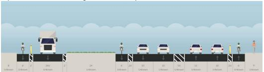
Orms St from Charles St to 100 ft to the west (the project boundaries for Capital Improvement Program work) should be restriped to eliminate one vehicular travel lane and install separated bike lanes on each side, as pictured below:
