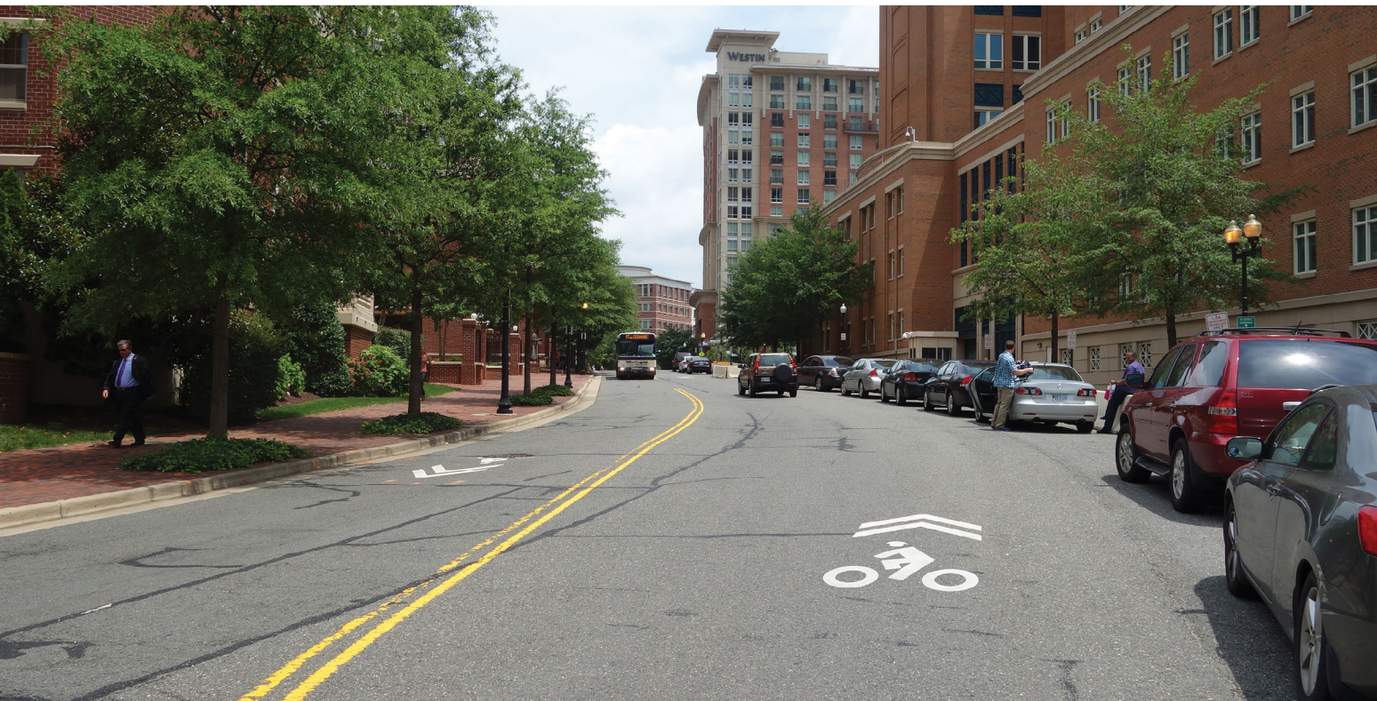
Shared Lane Marking Marcas de Carril Compartido
