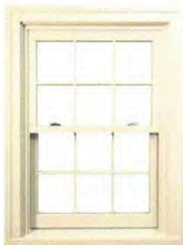
EC300 SHOWN IN BEIGE WITH OPTIONAL 3 1/4" WILLIAMSBURG BRICKMOULD, 1 1/4" HISTORIC SILL AND 1/2" SDL GRILLE.
