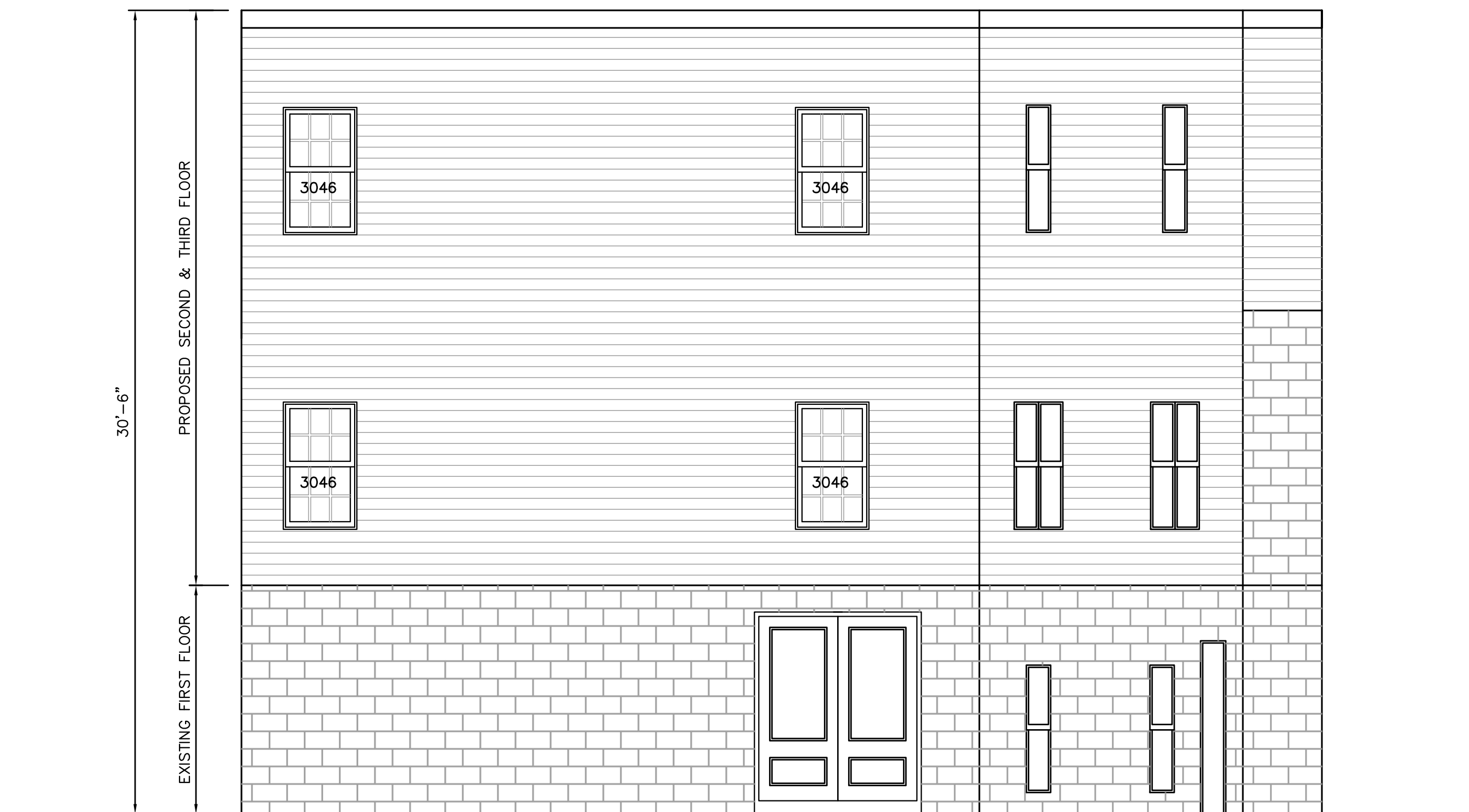
PROPOSED REAR (NORTH) ELEVATION SCALE: 1/4"=1'-0"
