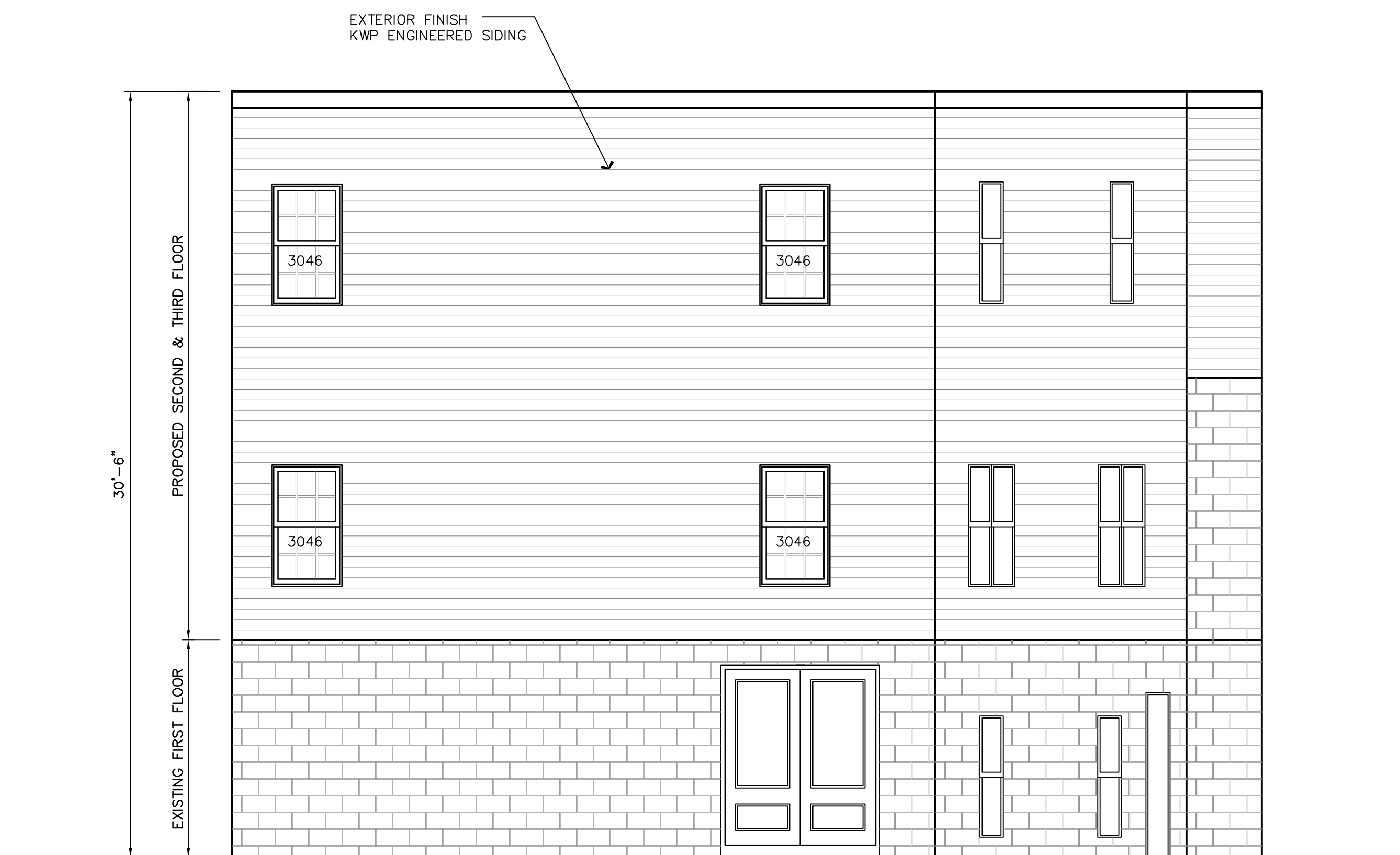
PROPOSED REAR (NORTH) ELEVATION SCALE: 1/4"=1'-0"
