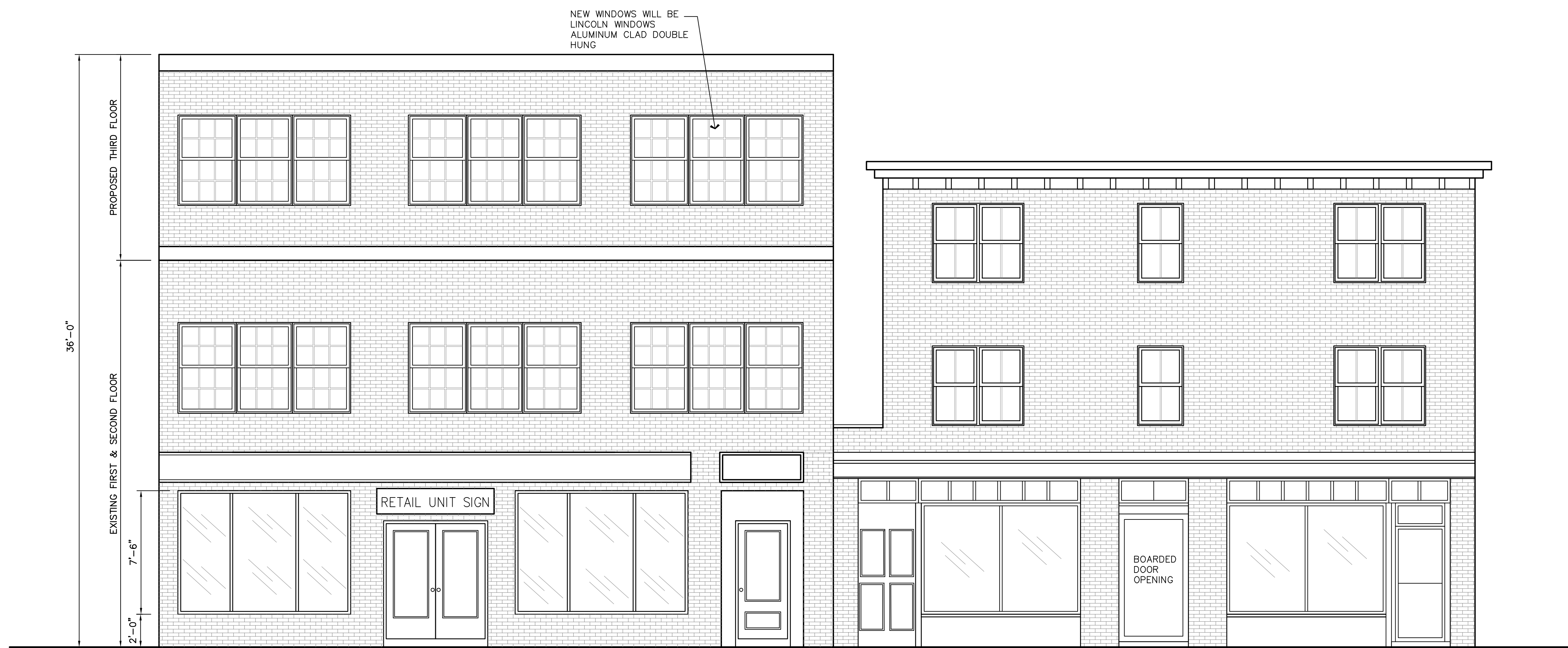
PROPOSED FRONT (SOUTH) ELEVATION SCALE: 1/4"=1'-0"
