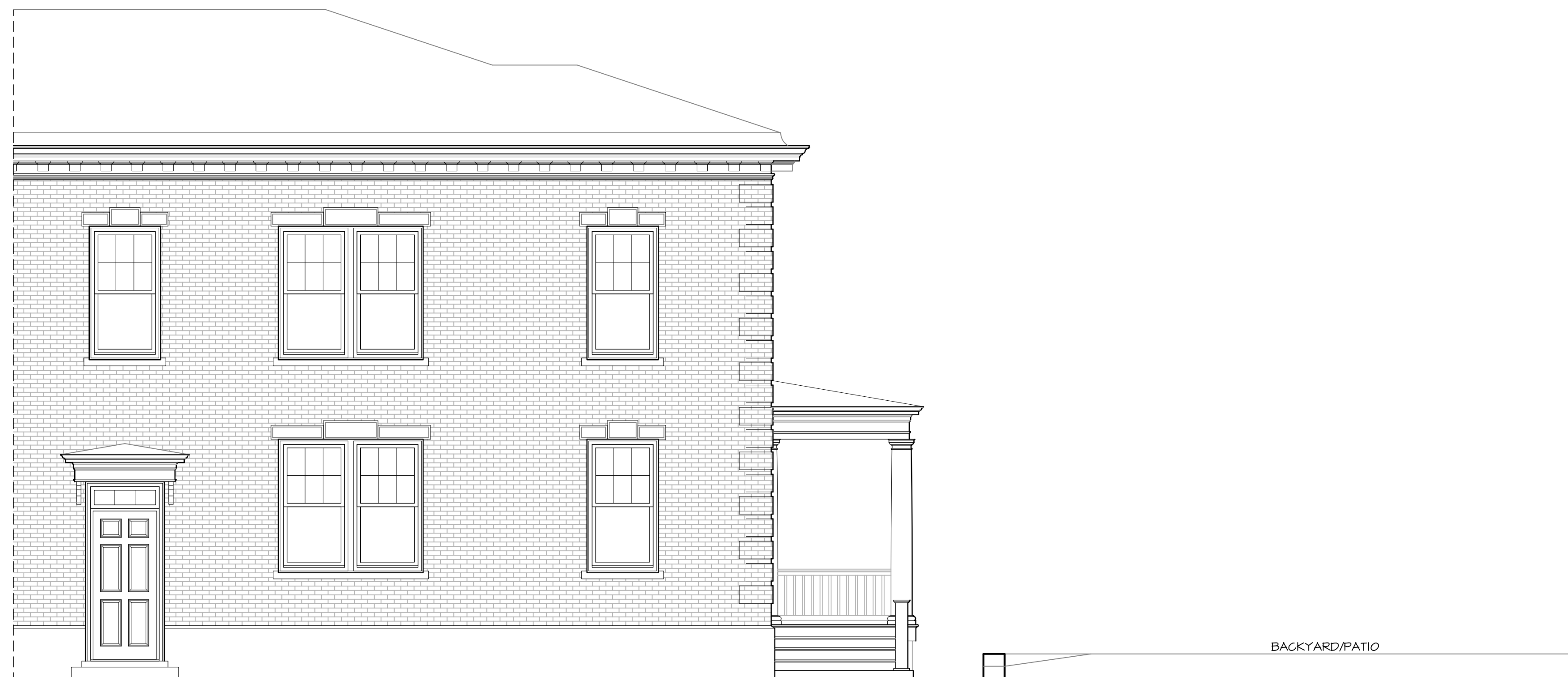
B EXISTING EXTERIOR ELEVATION, EAST SCALE: 1/4" = 1'-0"
