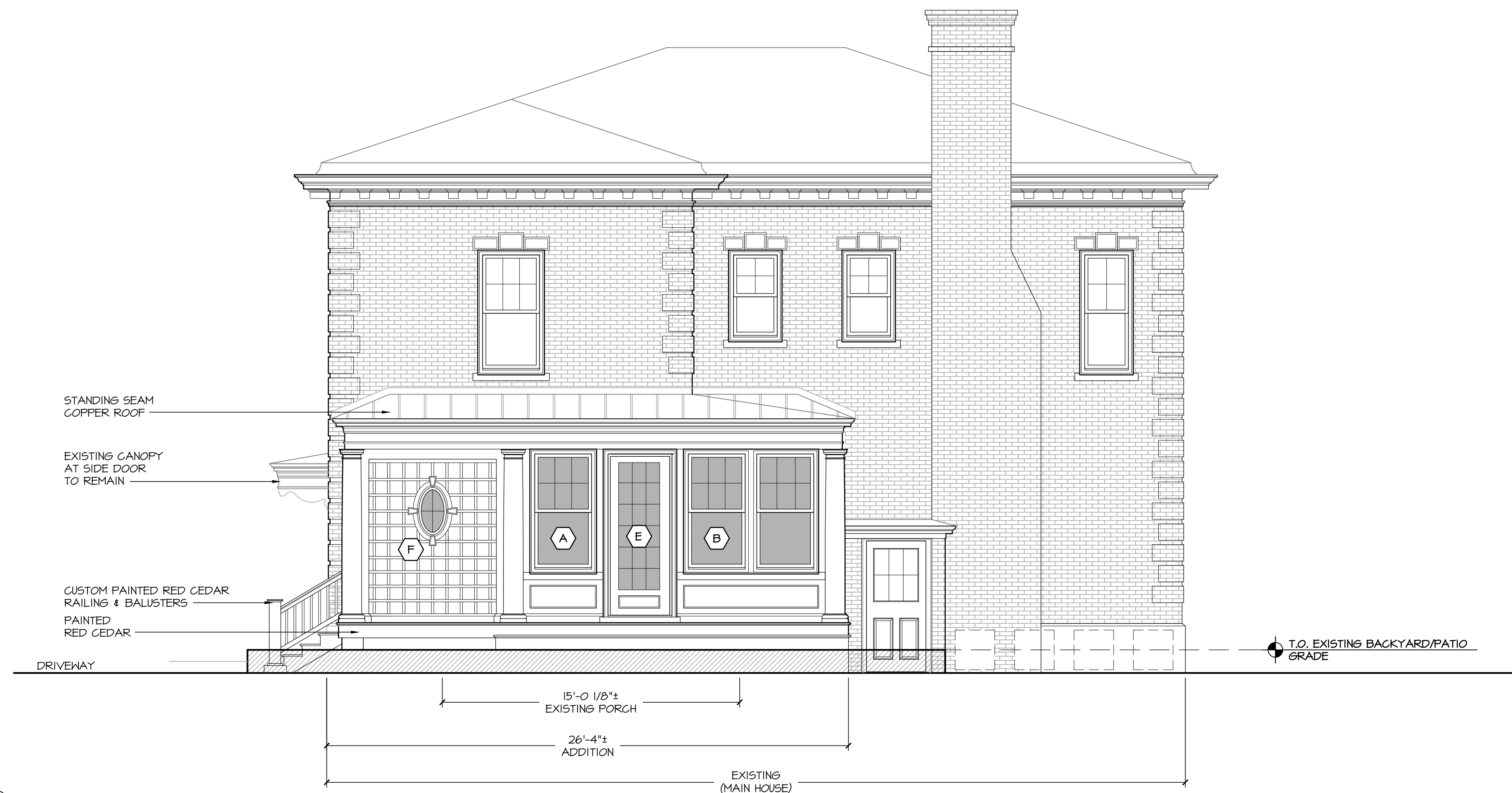
A EXISTING EXTERIOR ELEVATION: NORTH SCALE: 1/4" = 1'-0"
