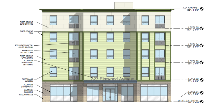
3-5 EXTERIOR ELEVATION - EAST (ELMWOOD AVE.) 1" = 1'-0"
