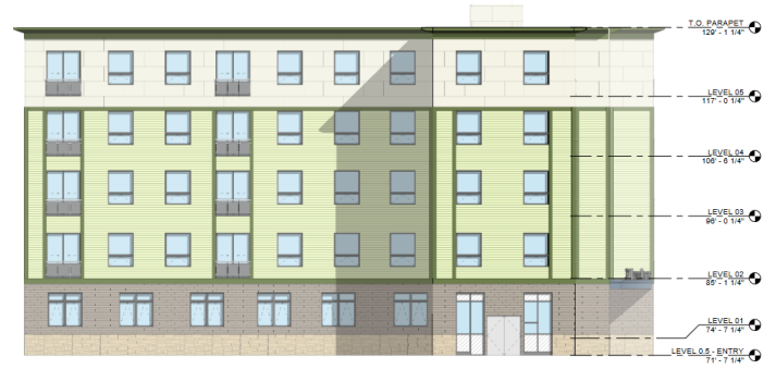
3-5 EXTERIOR ELEVATION - SOUTH (BURNETT ST.) 1" = 1'-0"
