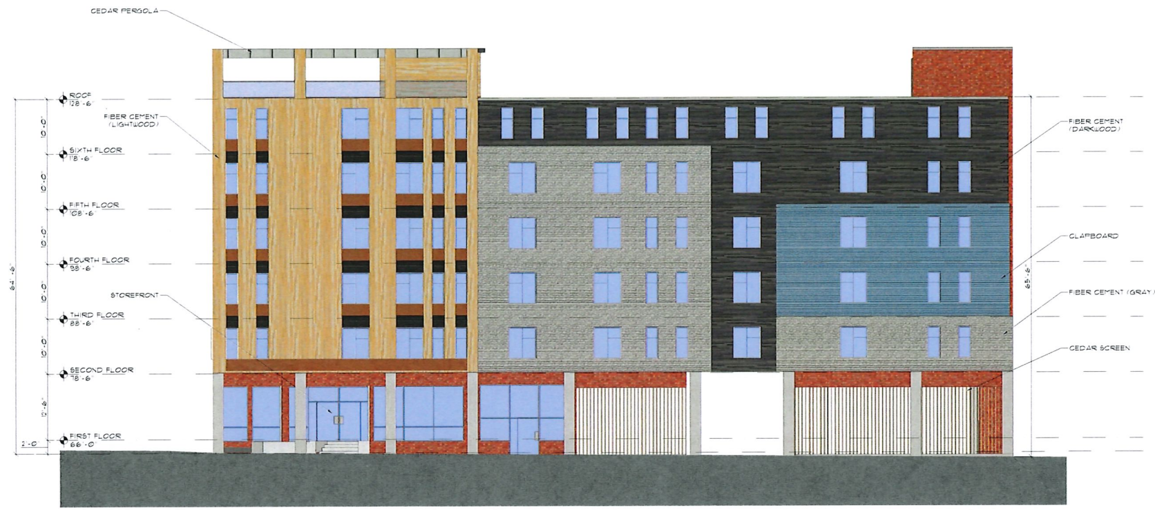
NORTH ELEVATION - WASHINGTON STREET (1) 3/32" = 1'-0"
