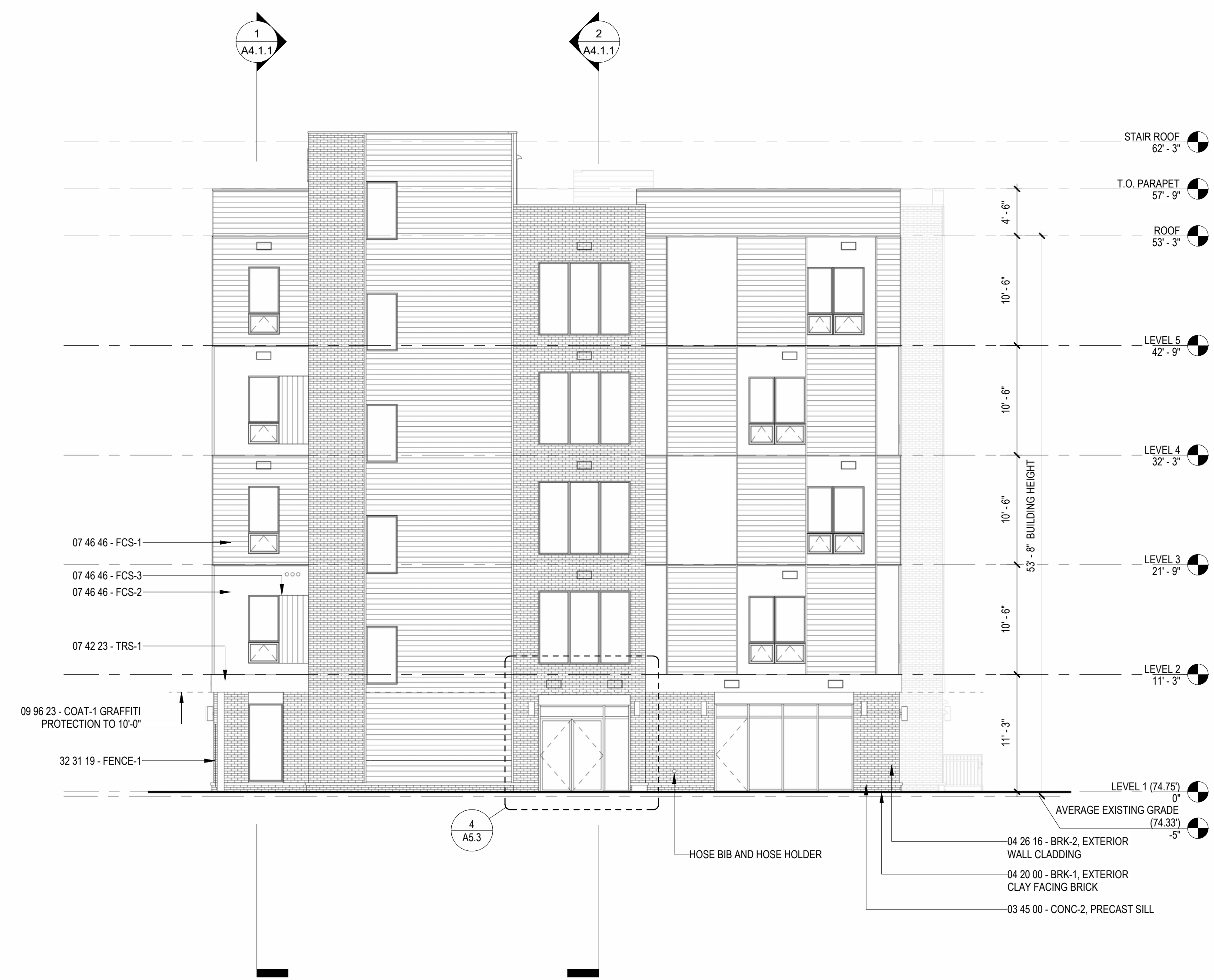
1 BUILDING ELEVATION EAST ELEVATION | 1/8" = 1'-0"
