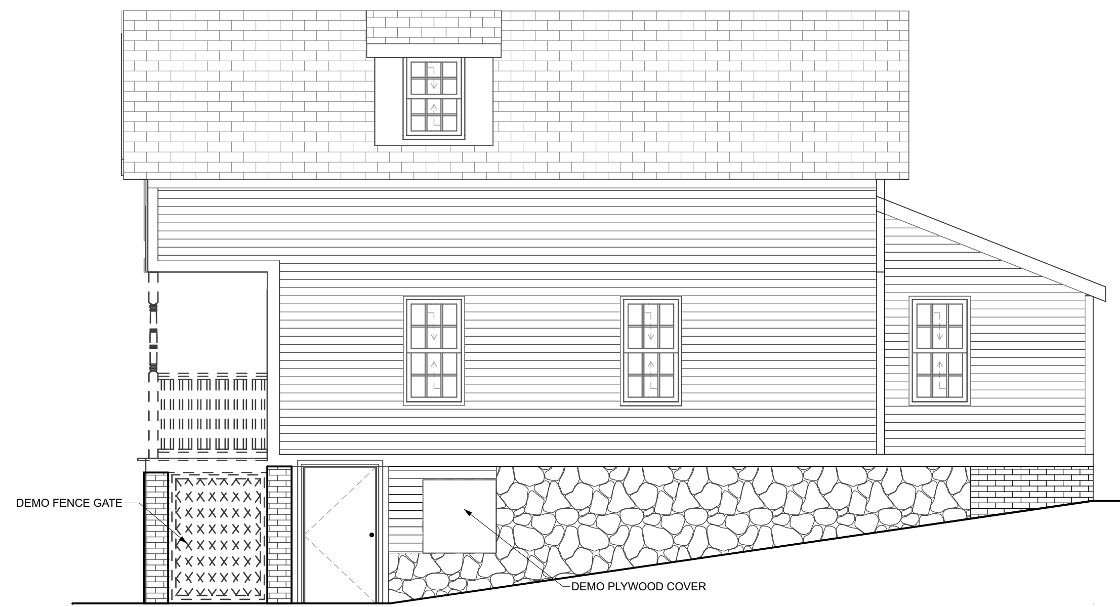
D1 EAST DEMOLITION ELEVATION
