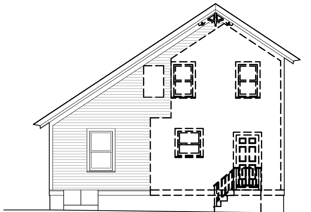
3 NORTH ELEVATION SHOWING DEMOLITION SCALE: 1/8" = 1'-0"
