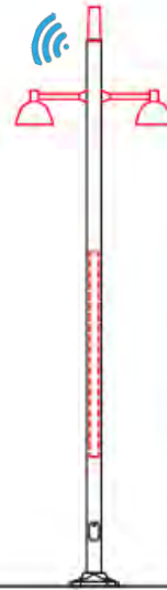
Pedestrian Post with Twin Pathway Luminaires
