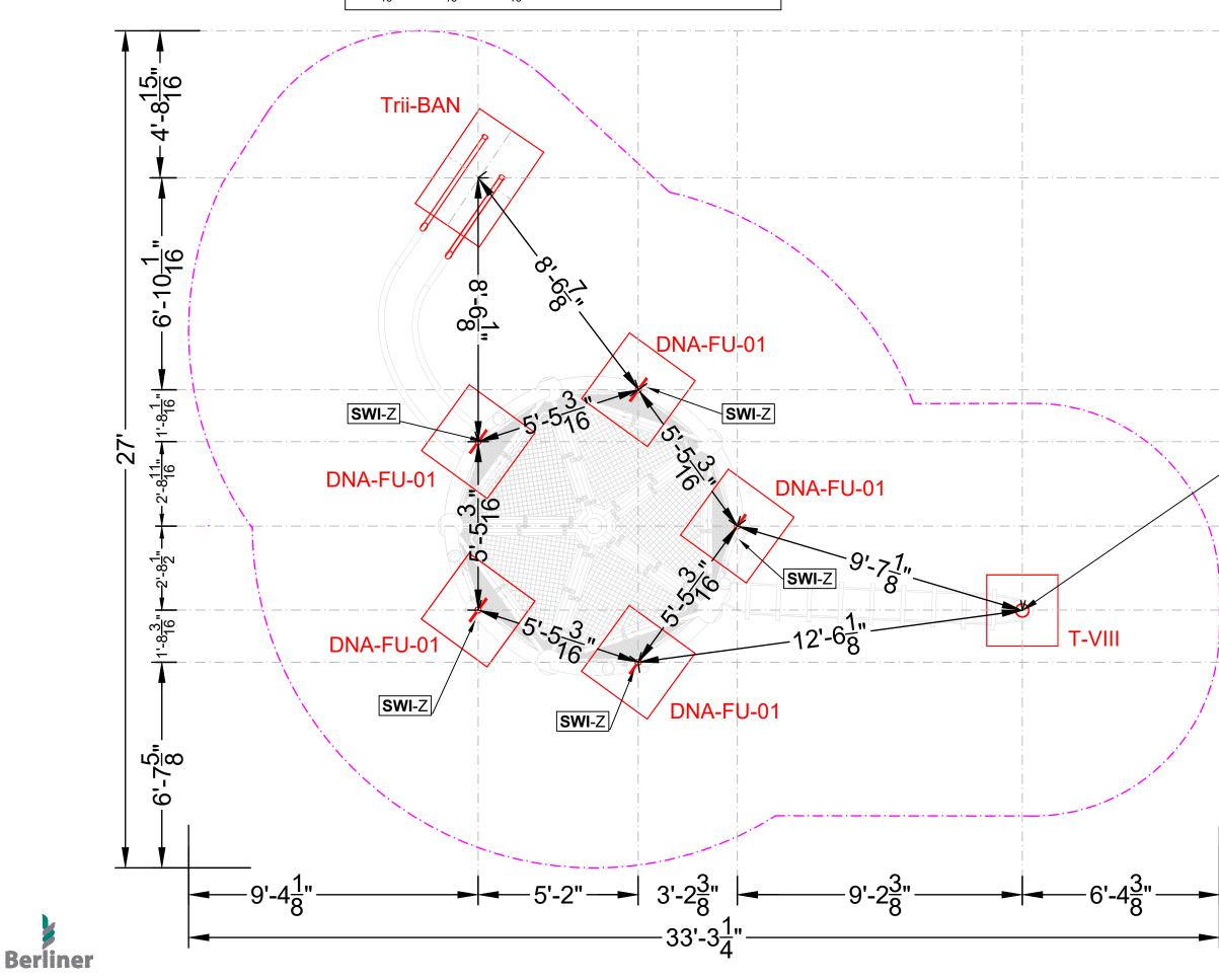
Fundamentlehre/foundation frame: 5x FU-Rohr/tube Ø60,3x10,0x825mm /  $\emptyset 2 \frac{3}{8} x_8^3 x_2^3 x_2^3 x_2^3$ 5x Rohr/tube Ø48,3x3,2x1422mm Ø1 <sup>7</sup>/<sub>8</sub>".<sup>1</sup>/<sub>8</sub>".4'-8" 5x Kugel/ball SWI-Z
