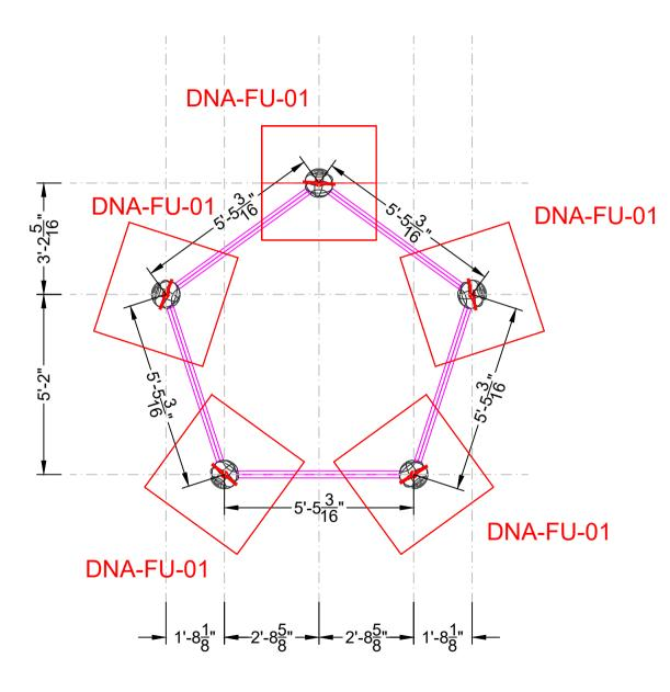
Fundament/Foundation **DNA-FU-01** 1100x1100x700mm/ 3'-7  $\frac{5}{16}$ "x3'-7  $\frac{5}{16}$ "x2'-3  $\frac{9}{16}$ "
