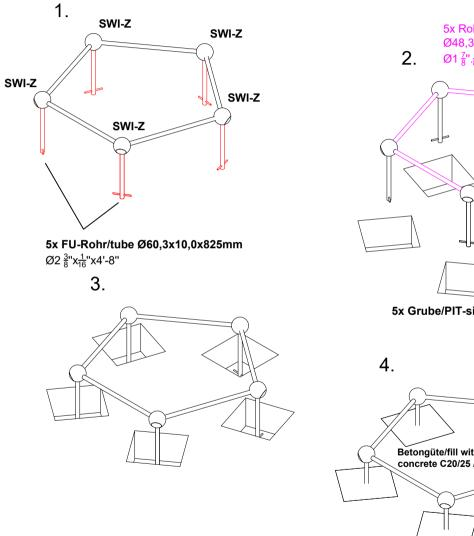
5x Rohr/tube Ø48,3x3,2x1422mm Ø1 <sup>7</sup>/<sub>8</sub>".<sup>1</sup>/<sub>8</sub>".4'-8'
