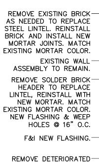
LINTEL AND REPLACE WITH NEW GALVANIZED STEEL LINTEL. MATCH EXISTING GUAGE & DIMENSION.
