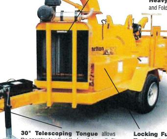
**30" Telescoping Tongue** allows the operator to adjust the length to easily fit under the largest chip bodies.
