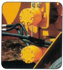
**32 Cubic Inch Feed Wheel Motors** give the Carlton 12" Chippers more infeed pulling power than any other 12" capacity chipper on the market. The patented coupler design makes the infrequent service extremely easy.
