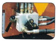
Integrated Single Manifold Hydraulic System simplifies the system reducing the number of hoses needed and reduces leak points.
