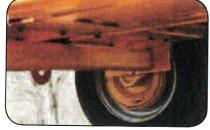
**8000 lb. Dexter Torflex Axle** with electric brakes makes Carlton 12" Chippers tow great. A 9000 lb. axle is used on the HD models.
