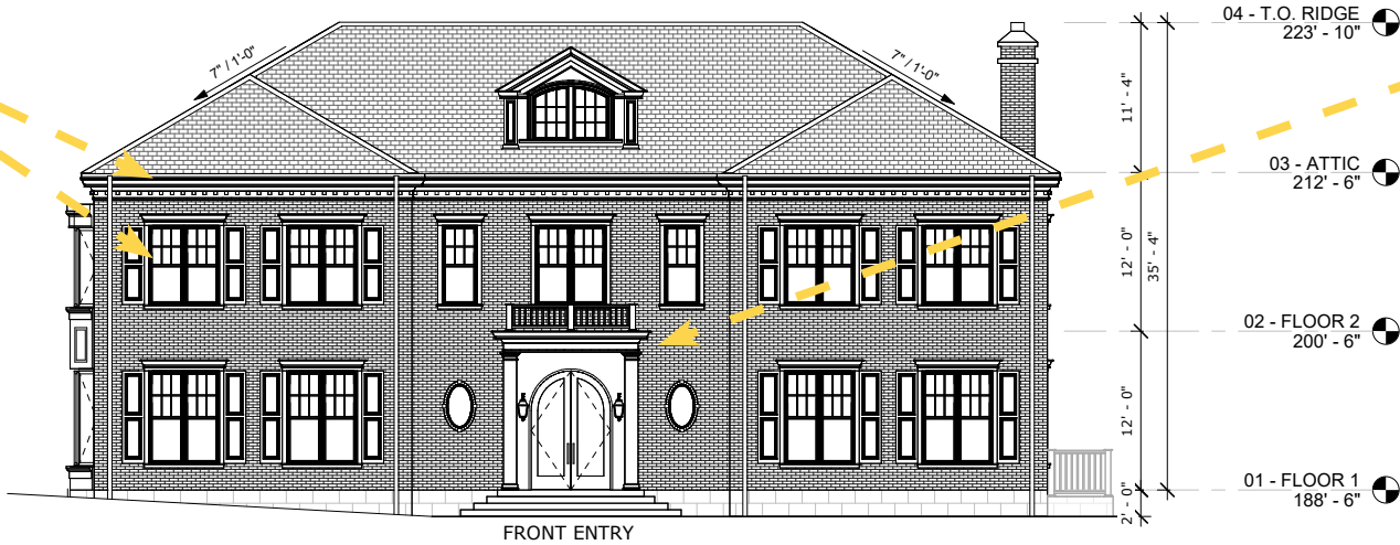
③ EAST ELEVATION - PROSPECT STREET 1/8" = 1'-0"
