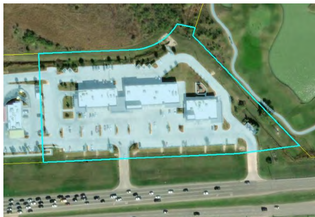
Figure 13. Example of non-residential property with captured impervious area (in light blue)
