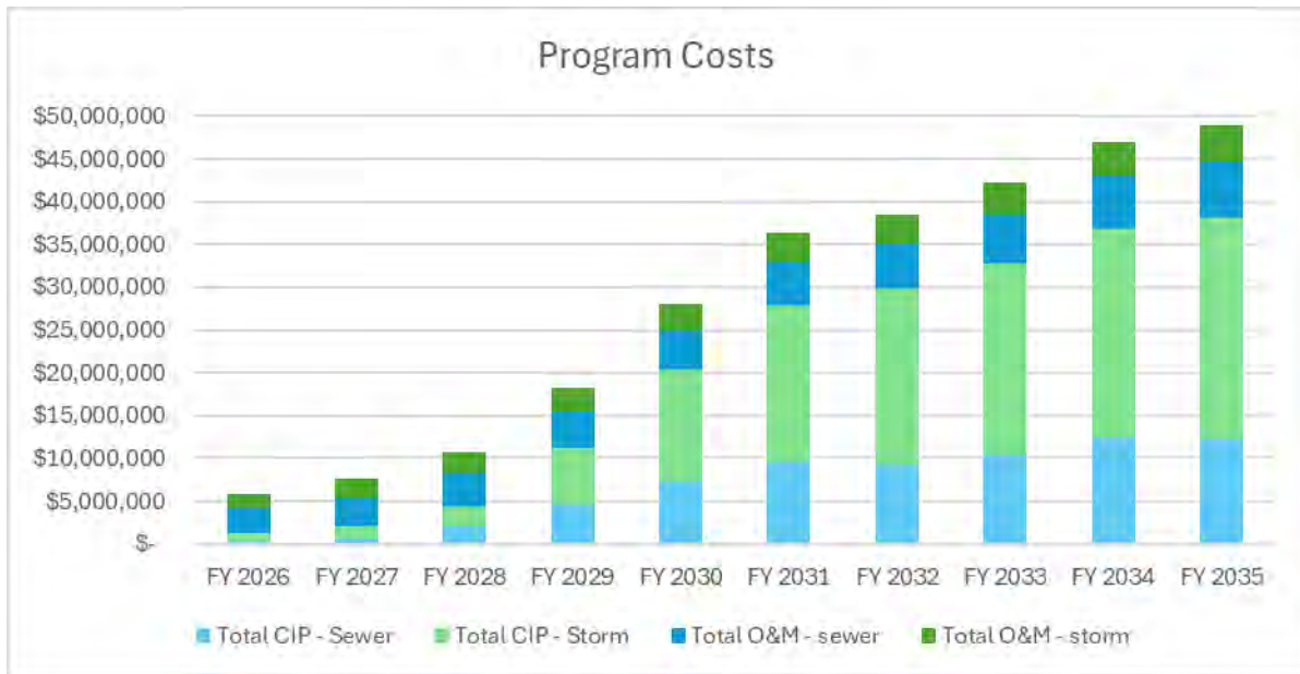
Figure 2: Sewer and stormwater estimated program costs by category for 10-year planning period
